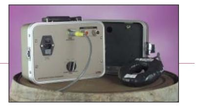
The Arbiter Systems<sup>®</sup>, Inc. Model 936A Reference Current Transformer provides laboratory grade accuracy in a small, portable, ruggedized case, making it ideal for field use. Multiple ratios of 1200:5, 1000:5, 800:5, 600:5 are selectable via a front panel switch. The guaranteed accuracy over the full input range and operating conditions is 0.02% ratio and 0.01° phase (traceable to NIST), ideal for calibrating other current transformers.
